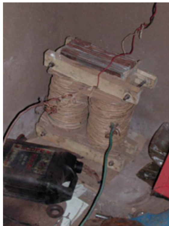
Nyamyotsi I (Rwanda): Productive use (locally produced welding transformer)
